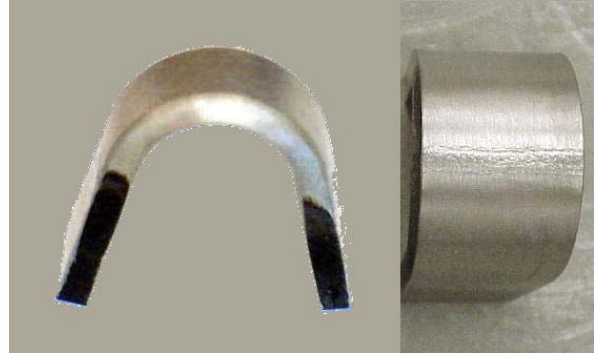
Figure 8: Bend test of a butt weld specimen
